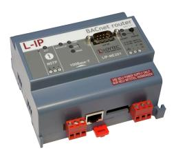
The LIP-ME201 BACnet/IP Router connects a BACnet MS/TP channel to a BACnet/IP network. It routes BACnet packets back and forth through an IP based network, such as a LAN (Ethernet), an Intranet, or even the Internet. The LIP-ME201 is compliant with the standards ASHRAE 135-2008 and ISO 16484-5. LIP-ME201 can be configured to act as a BACnet Broadcast Management Device (BBMD). The L-IP also provides Foreign Device support. For MS/TP slave devices, the router acts as a Slave Proxy.
